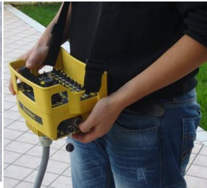
Emergency push button pendant (electric) on board of the machine
