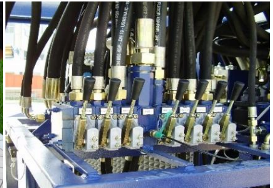
Emergency proportional hydraulic distributor (manual)
