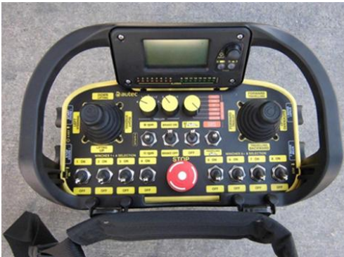
Remote control (electric) with electro-proportional commands
